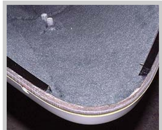
HDPE behind the lip of the hull where the stainless screws will bite
