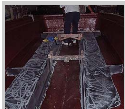
Stringer System being installed
