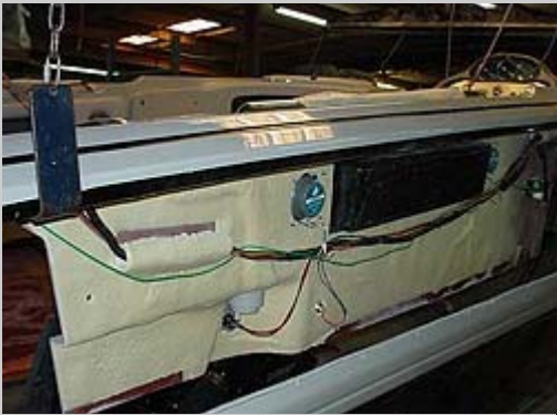
Deck about to be set into a hull
