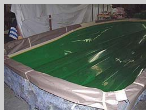
Taped off mold before getting sprayed
