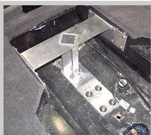
Super reinforced direct drive pylon bracket
